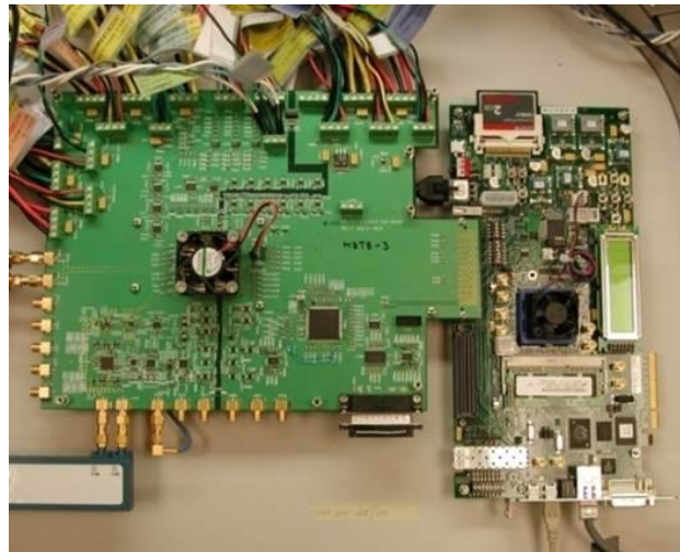
Figure 3-16: Development platform with digitizer board (left) and ML605 board (right)
