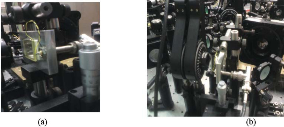
Fig. 2 (a) Picture of the q-plate mounting. Both the q-plates adopted have been controlled by an electric field, applying a voltage to the liquid crystal. (b) Motorized waveplates in order to generate/analyze different states in an automatic way.
