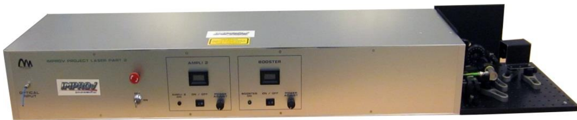
MULTITEL first amplifier with the 25 \mu\text{m} step-index fibre.
