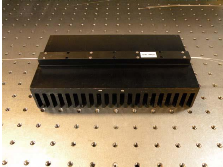
Passive PCF-combiner placed on a heat sink
