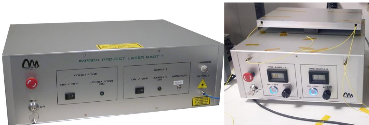
MULTITEL gain-switch laser prototype (left) and amplifier with pulse stretchers (right).
