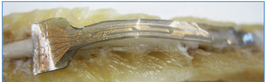
Figure 1: Our first FMEA with 6 electrodes on a rat spinal cord. The square-shaped contact pads are visible on the left and connected to the electrodes ( \varnothing 200 \mu m) via intersecting serpentine traces that provide greater elasticity than straight traces.
