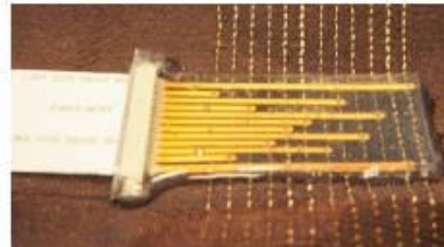
Stretchable interposer to connect textile electronics with environment
