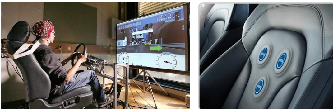
Figure 16 Measuring the brain activity [Nissan] or the heart rate [Plessey] of the driver
