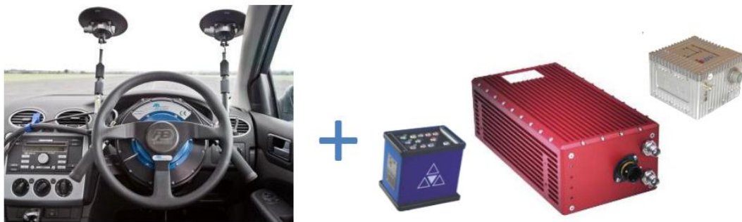
Figure 17 Steering robot (ABD) and GPS (OxTS, GeneSys, or iMAR)
