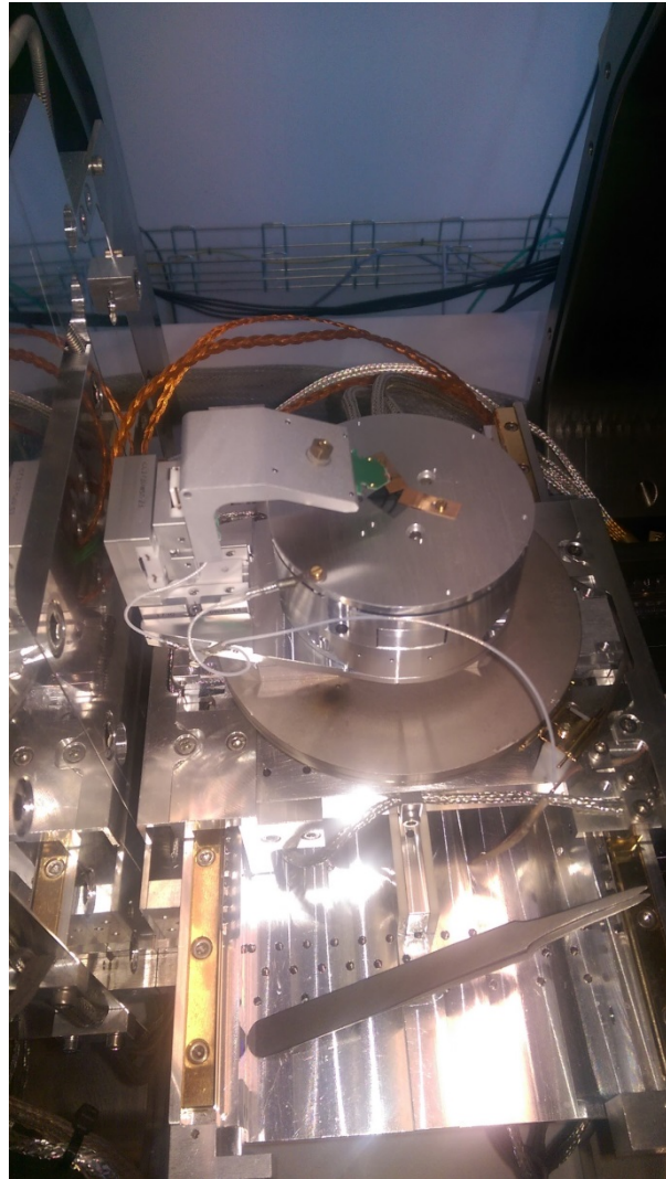
Fig. 1 The AFM as mounted on the stage of the FEI NovaNanoLab650 SEM
