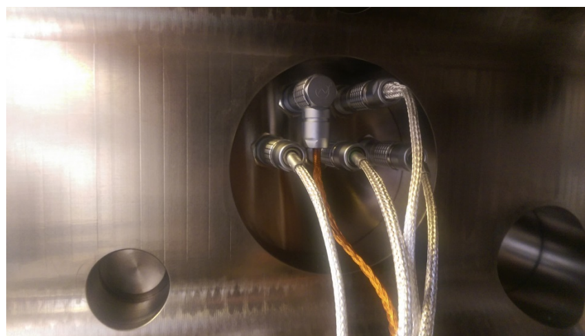
Fig. 2 The vacuum side of the flange containing the AFM electrical feedthroughs.
