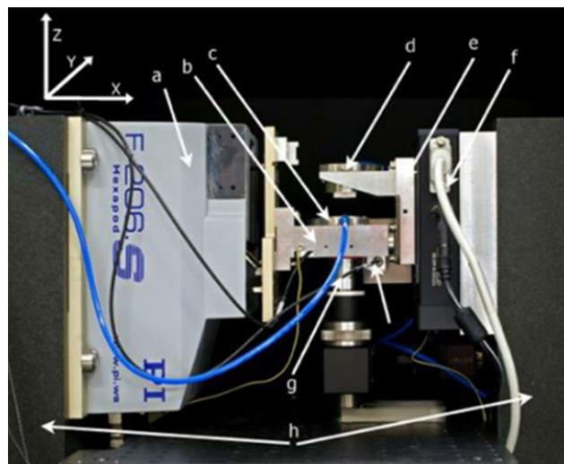
**Fig. 18** The 6D-alignment tool. a) the 6D-stage (PI F206 hexapod), b) 6D-stage mounting fork, c) lower element chuck, d) upper element chuck, e) z-stage mounting fork, f) z-stage (PI M605-1D), g) microscope objective, h) granite stage mounting blocks.
