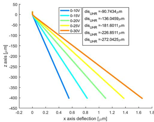
**Fig. 33** Particle trajectories (of the central beam) beyond the blanker when the micro deflector (at z=0) is switched on (voltages in the range 10V-30V on one electrode, 0V on the other)
