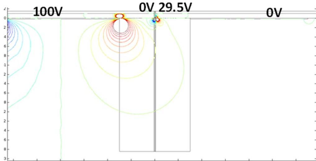
**Fig. 30** COMSOL simulation of the electrostatic fields due to the indicated voltages on the micro and macro deflectors. The equi-field strength lines are shown
