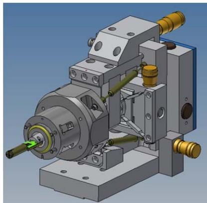
**Fig. 22a** A schematical drawing of the chip stack support assembly.
