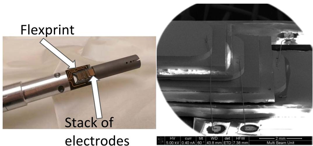
**Fig. 20** Left: part of the flex print is seen next to the rear of the electrode stack. Right: SEM image of the wire bonds between the electrode stack and the contact pads of the flex print.
