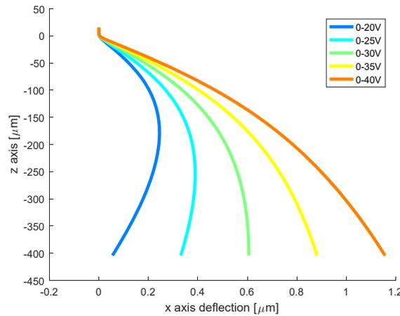
**Fig. 35** Macro deflector: -50V -> +50V (symmetric); Micro deflector indicated in legend (asymmetric). When 0V->30V are applied, the beam direction remains vertical.
