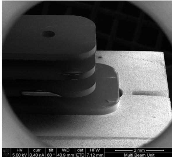
**Fig. 19** An SEM image of the beam splitting optics stack, consisting of 3 macro-electrodes (on top) and the MLA (bottom).
