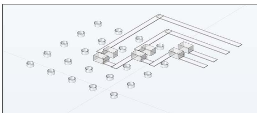
**Fig. 13** Design of the deflector electrodes on the blanker plate, in the prototype configuration with 3 micro electrodes only.
