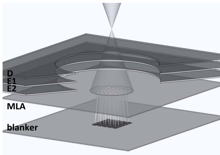
**Fig. 4** Cross-section of the Multi Beam Blanker Unit
