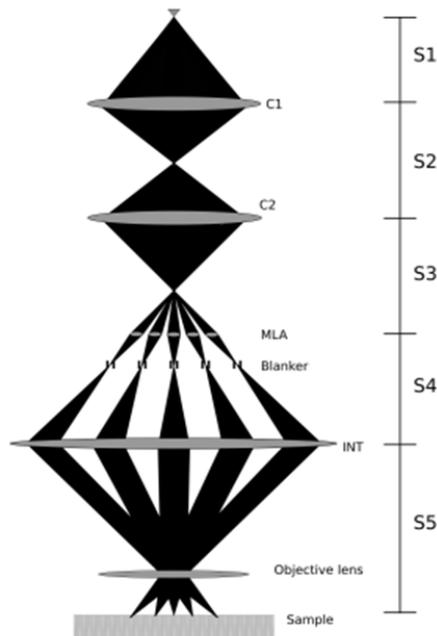
**Fig. 9** The optical column is divided into five segments for which the statistical Coulomb interactions are calculated.
