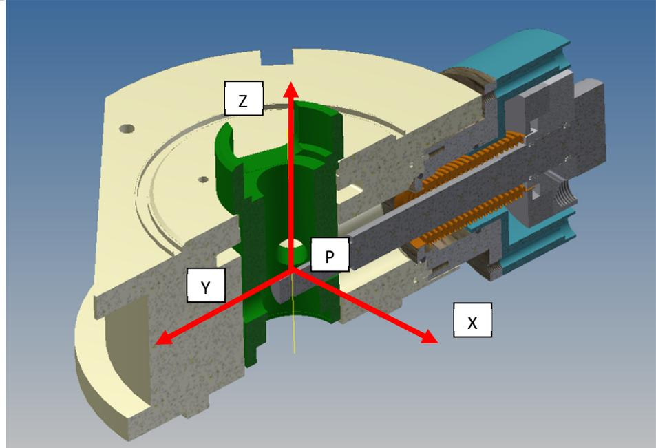
**Fig. 21** Definition of the axis system
