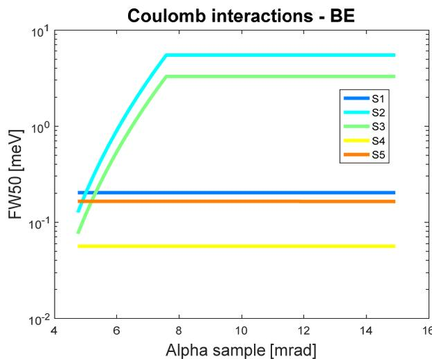
**Fig. 11** The Full-width containing 50% of the energy distribution due to the Boersch effect.
