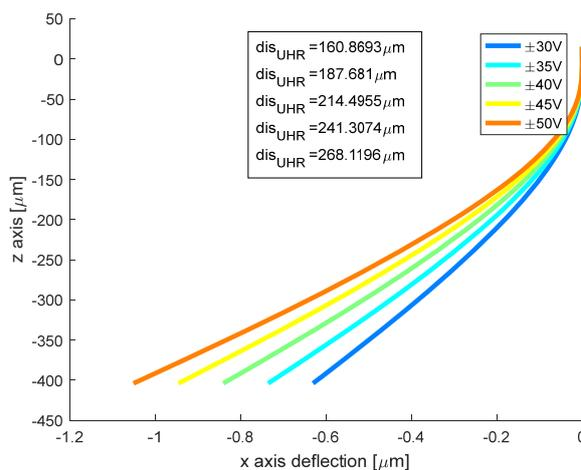
**Fig. 31** The deflection as a function of the distance towards the macro deflector, located at  $z=0$ . The displacement of the trajectories in the UHR lens plane are indicated in the inset for the indicated voltages ranging from 30-50 V, applied symmetrically to both electrodes.
