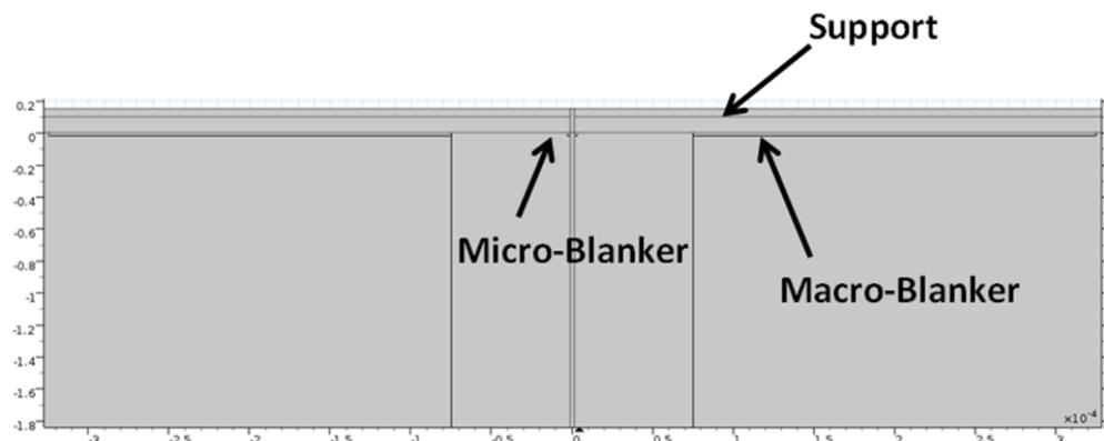
**Fig. 29** COMSOL geometry to simulate the deflection angles of the micro and macro deflectors.
