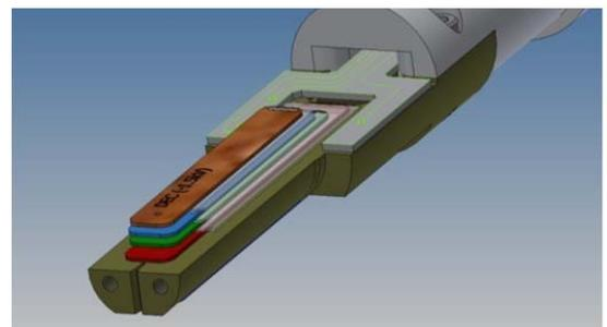
**Fig. 22b** Schematical drawing of the support with the chip stack mounted on top.
