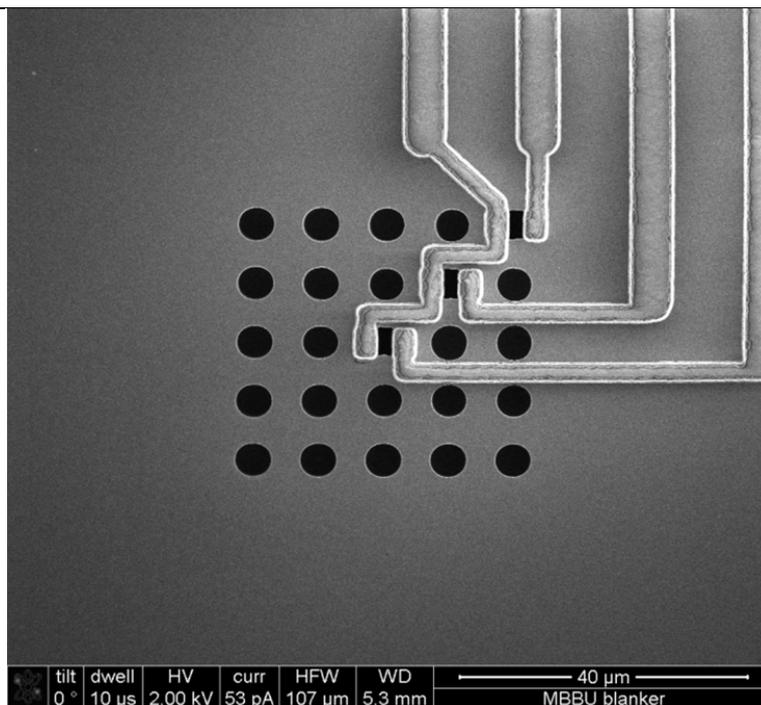
**Fig. 38** SEM image of the micro electrodes defined around three of the 25 holes in the deflector array plate. The macro electrodes are at a larger distance from the array, outside of the field of view in the image.
