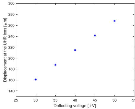
**Fig. 32** Deflection of the central beam when the macro blanker is active with the indicated deflecting voltages.
