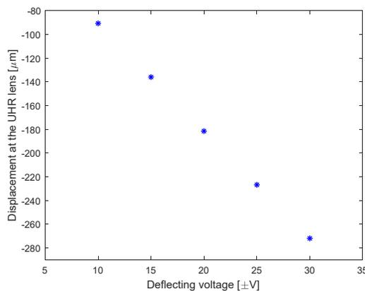
**Fig. 34** Deflection of the central beam when the micro blanker is active with the indicated deflecting voltages.
