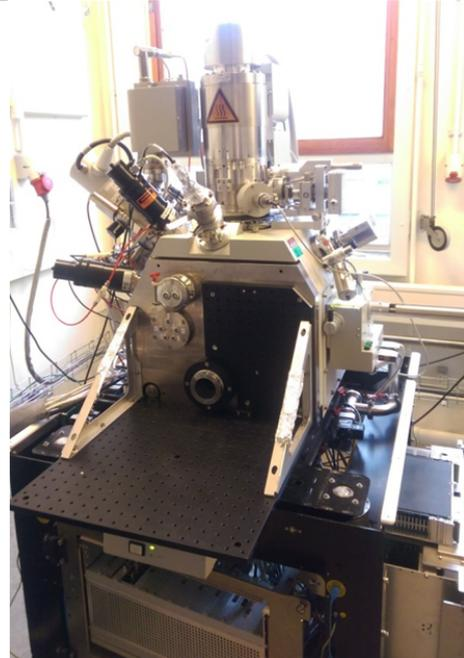
**Fig. 26** Left: schematic of the SECOM platform mounted in an SEM. Right: View at the SECOM platform mounted in the SEM. Also seen is the chip stack assembly mounted in the variable aperture port on the lower right side of the column.
