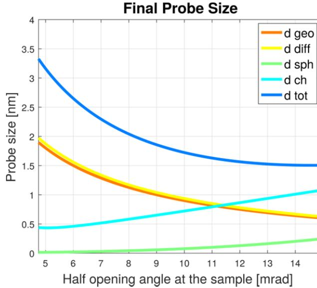
**Fig. 5** Variation of the total axial probe size and the on-axis aberration contributions to the probe as a function of the beam half opening angle at the sample
