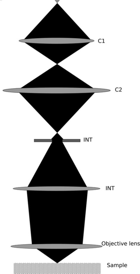
**Fig. 2** Optical schematics of an electron microscope in single beam mode
