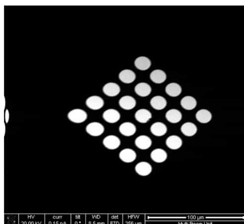
Fig. 25 Cross-over mode image of the MLA, detected using the Everhart Thornly Detector, the standard SE-detector.
