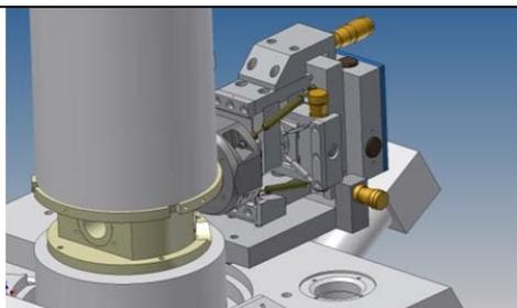
**Fig. 22c** Schematic drawing of the assembly mounted to the SEM column.
