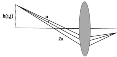
**Fig. 6a** Off axis beam focused on the image plane by a lens
