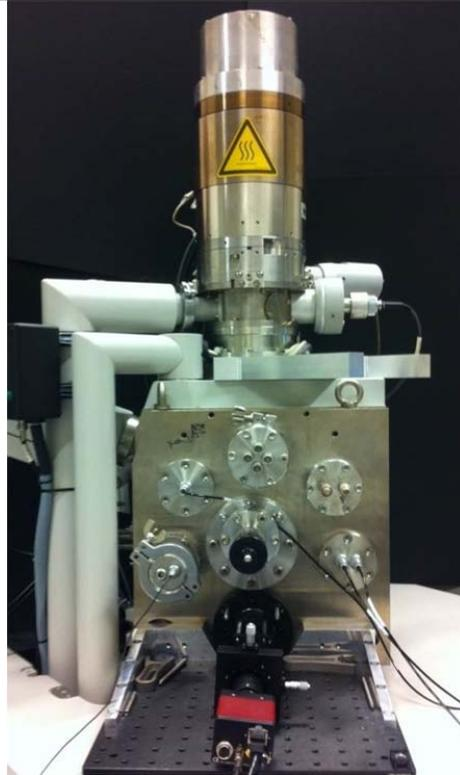
**Fig. 1** The Multi Beam Scanning Electron Microscope (MBSEM) with 196 beams.
