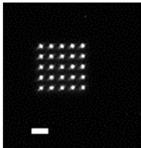
**Fig. 27** Optical image of the 25 beams focused on a YAG screen. The scale bar is 10  $\mu\text{m}$ .
