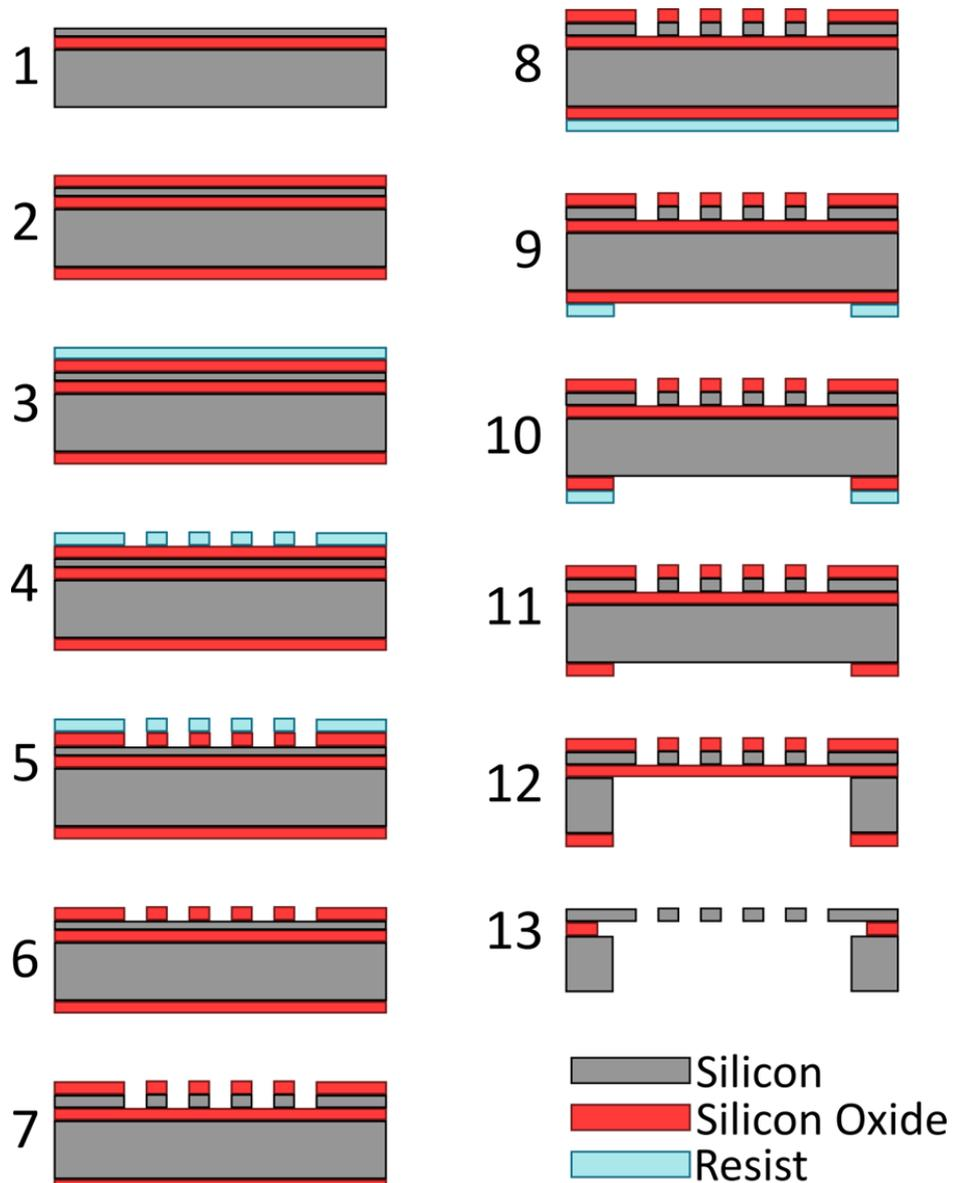
Fig. 16 Schematic overview of the process steps in the fabrication of the Micro Lens Array (MLA).
