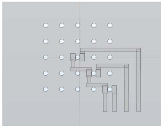
**Fig. 28** Top view of the three micro deflectors. The distance between the electrodes is  $2.5\mu\text{m}$ , and the width of the connecting leads is  $2\mu\text{m}$ .
