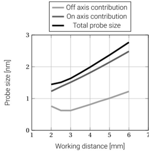
**Fig. 8** On-axis and off-axis contributions to the probe size and total probe size at the sample for different working distances.
