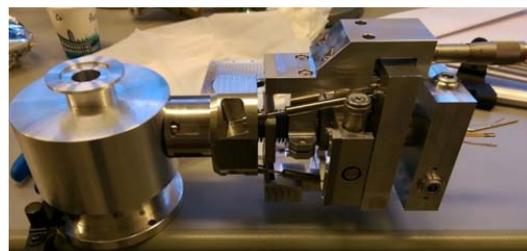
**Fig. 22d** The assembly mounted to a test part resembling the SEM column.
