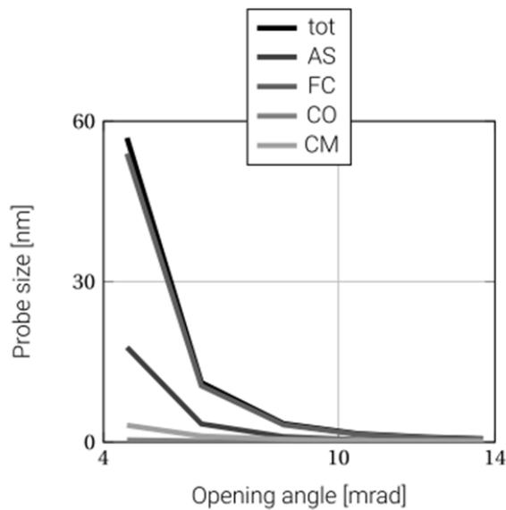
**Fig. 7** Off axis contributions to the probe size and total probe size at the sample for different half opening angles of the beams at the sample.
