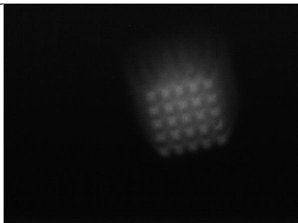
Fig. 24 Shadow image of the MLA for the lens settings shown on the left.
