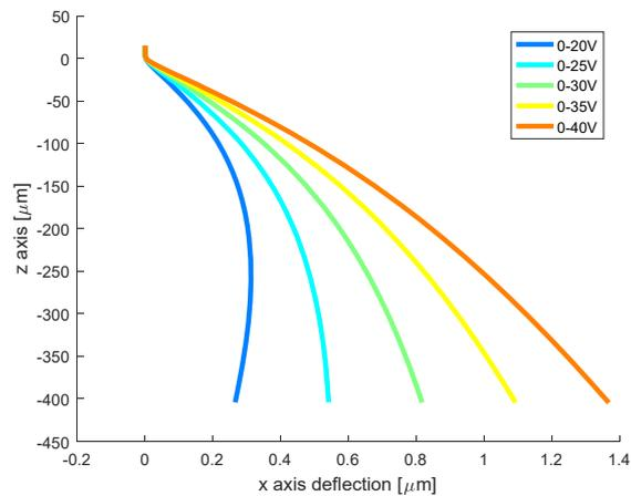
**Fig. 36** Macro deflector: -40V -> +40V (symmetric); Micro deflector indicated in legend (asymmetric). When 0V->25V are applied, the beam direction remains vertical.
