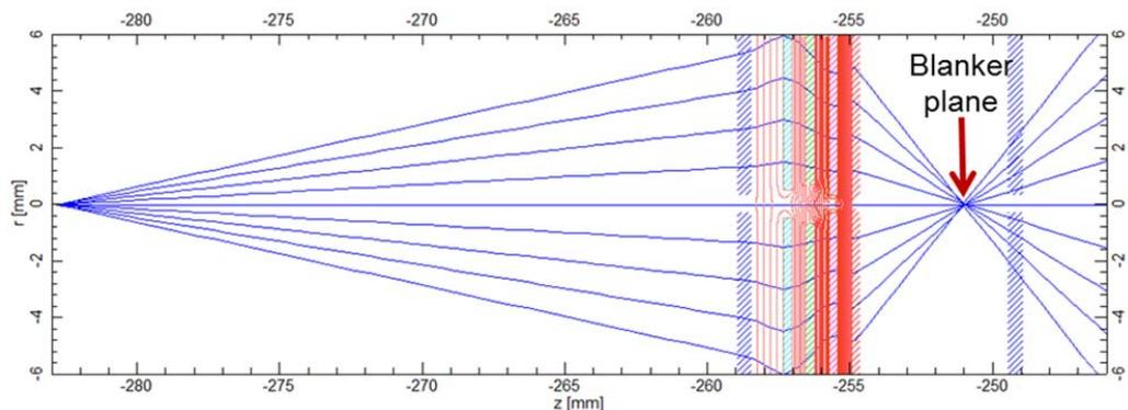
**Fig. 15** The equipotential lines of the calculated fields are shown in red between the electrodes, and the ray traces are shown in blue (not at the same scale as the geometry).
