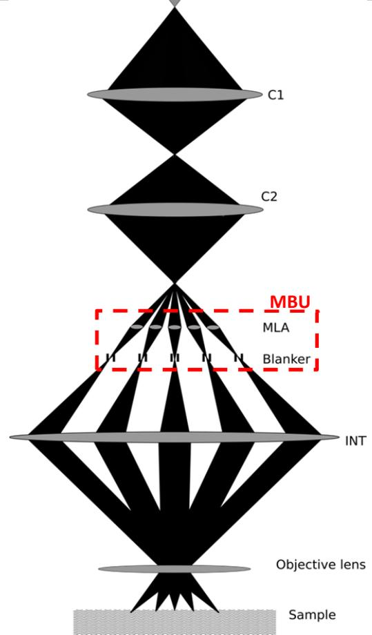
**Fig. 3** Optical schematics of an electron microscope in multi beam mode
