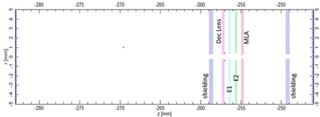
**Fig. 14** The electrode geometry of the beam splitting optics stack.
