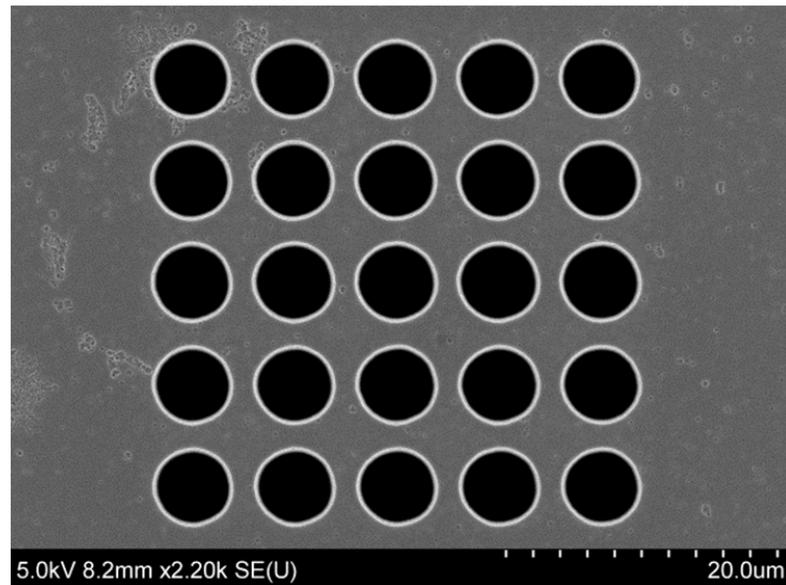
**Fig 17** An SEM image of the MLA. It consists of 25 aperture lenses of  $5 \mu\text{m}$  radius at a  $7.5 \mu\text{m}$  pitch etched out of a  $10 \mu\text{m}$  thick Si membrane.
