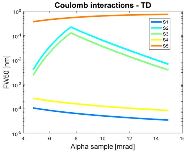
**Fig. 10** Probe size contribution due to trajectory displacement.
