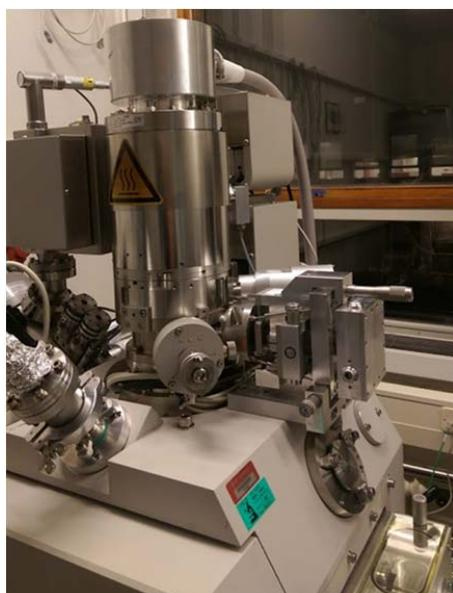
**Fig. 23** The chip stack support assembly mounted to the FEI NovaNanoLab SEM.
