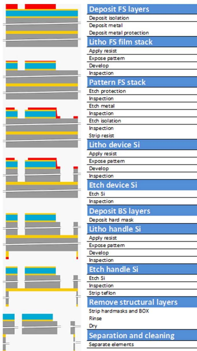
**Fig. 37** Process steps to fabricate the blanker array. The colours denote the following: grey: Si, yellow: oxide, blue: metal, red: resist.
