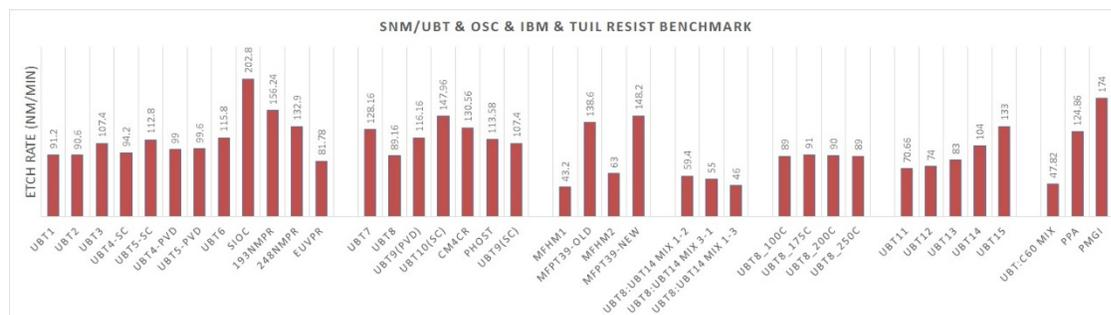
Figure 1: Etch rate overview of the different MG-platforms (UBTx, from UBT), Fullerene based resists (MFHM1/2 and MFPT39, from OSC), UBT/C60 mixture (from UBT/OSC), Calixarene (CM4CR, from TUIL), Polyphthalaldehyde and polydimethylglutarimide (PPA, PMGI from IBM) as well as the reference materials (SiOC, 193nm PR, 248nm PR and EUV-PR).
