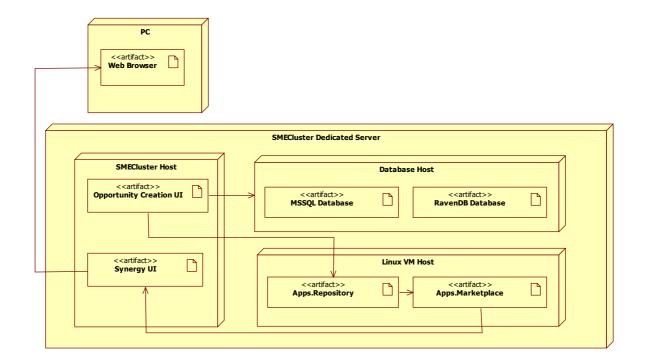
The network infrastructure is based on two development servers configured on a 100Mbps network located at the Control 2K headquarters at Waterton Centre. The network is TCP/IP based on IPv4 addressing using Dynamic Host Configuration Protocol. Server one will run
