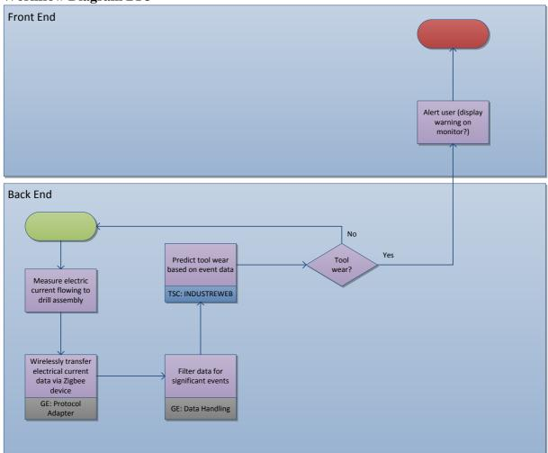
Predicting tool wear is important to a number of small manufacturers, as knowing in advance whether an assembly line is at risk of being disrupted is vital in a small business environment. This knowledge can then be used to plan to minimise disruption, or even to avoid it entirely.
