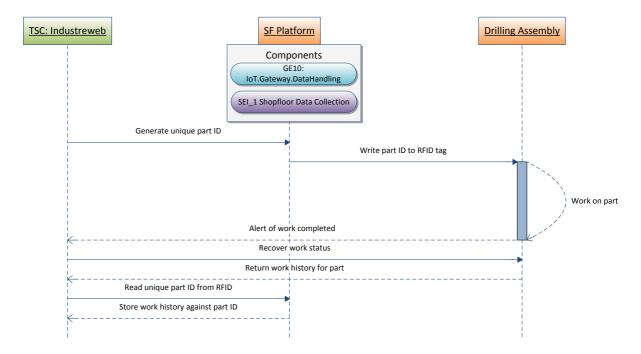
The RFID tag will be used to store a minimum of data, while Industreweb will store the work history of the part being worked on. Once the part's work is complete, the history will be combined with the part ID and stored to database.
