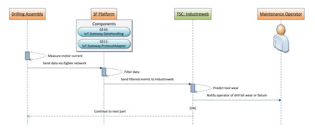
The drilling assembly draws an electrical current when working, whose value can be predicted. This value can then be used to identify the state of the drill bit, and to predict when it is approaching the end of its life, or a point at which it could produce sub-optimal results on the part it is working on.
