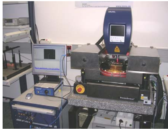
Figure 4: Measurement setup for single channel dynamic measurements (MSA500 and Cascade probe station)
