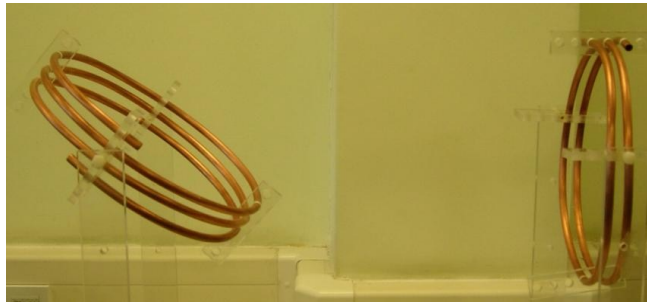
Figure 36: Misaligned 3 turn (left) and 2 turn (right) 30 cm diameter coils.
