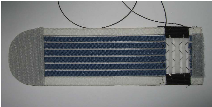
Figure 100 Second prototype of a tactile wristband with SMA actuators integrated into a monolithic structure
