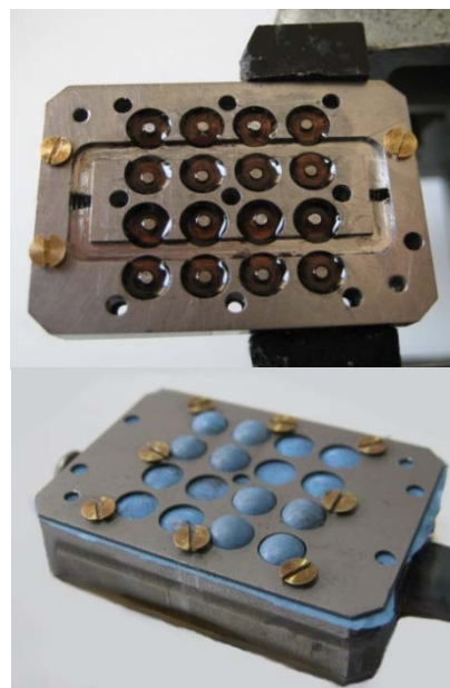
Figure 94 Supply channel with integrated coils and ferromagnetic core and on the bottom the assembled prototype
