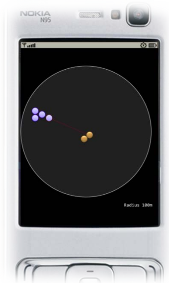
Figure 40 Screenshot of the visual component of FriendSense: direction and distance of all friends are shown in a radar-like UI. In the illustrated situation, two friends have strayed away from the group, which is to the left-hand side.
