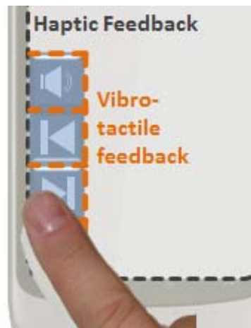
Figure 48 The basic concepts of the PocketMenu: the screens border and vibro-tactile feedback make the buttons "feelable".
