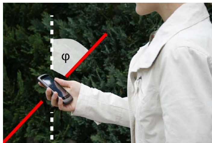
Figure 81 The detection of the device posture is done by using the integrated accelerometer.
