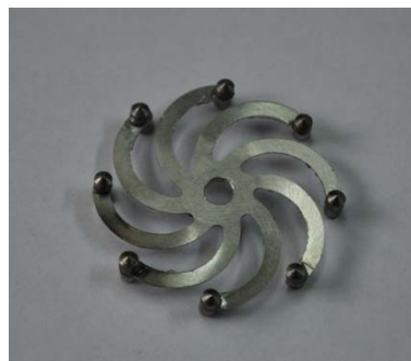
Figure 102 Monolithic structure with 8 lever beams
