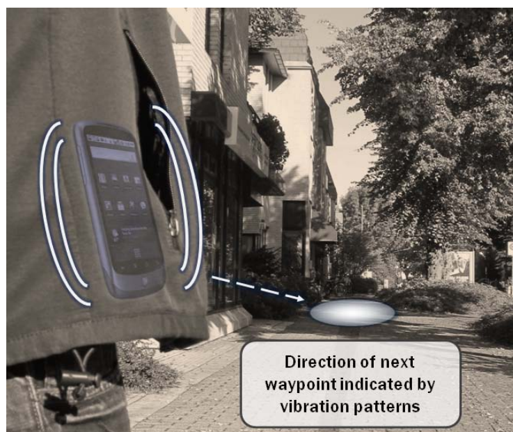
Figure 32 Vibration patterns indicate the direction of the next waypoint of a route.
