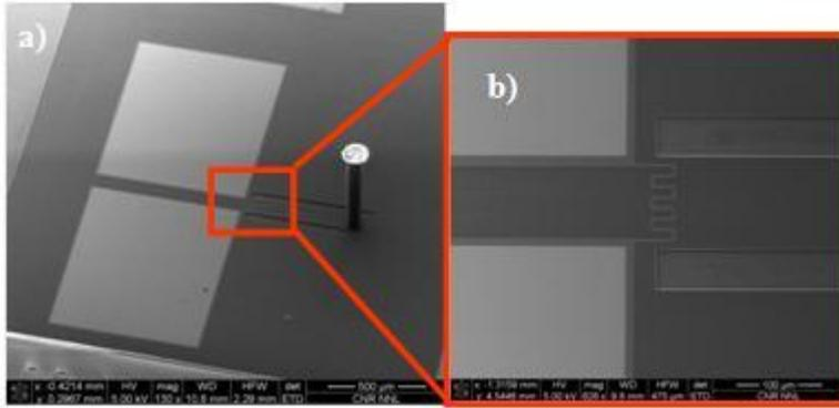
The flow sensor has an in-plane geometry with a Cilium on the free end of the cantilever. This cantilever is made in Silicon, using Silicon on Insulator (SOI) substrates. An original approach has also been proposed, which is under patent filing. More details will be given soon.
