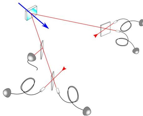
**Figure 1:** Entanglement distillation. The entanglement of a two-mode squeezed state is increased when an APD detects a single photon scattered by a weakly reflecting beam splitter in one arm. Weak-field homodyne detection with time-multiplexed detectors implements an efficient entanglement witness.
