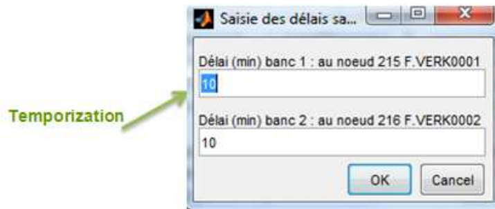
Figure 30: Changing parameters of reactive power regulation (capacitors banks)
