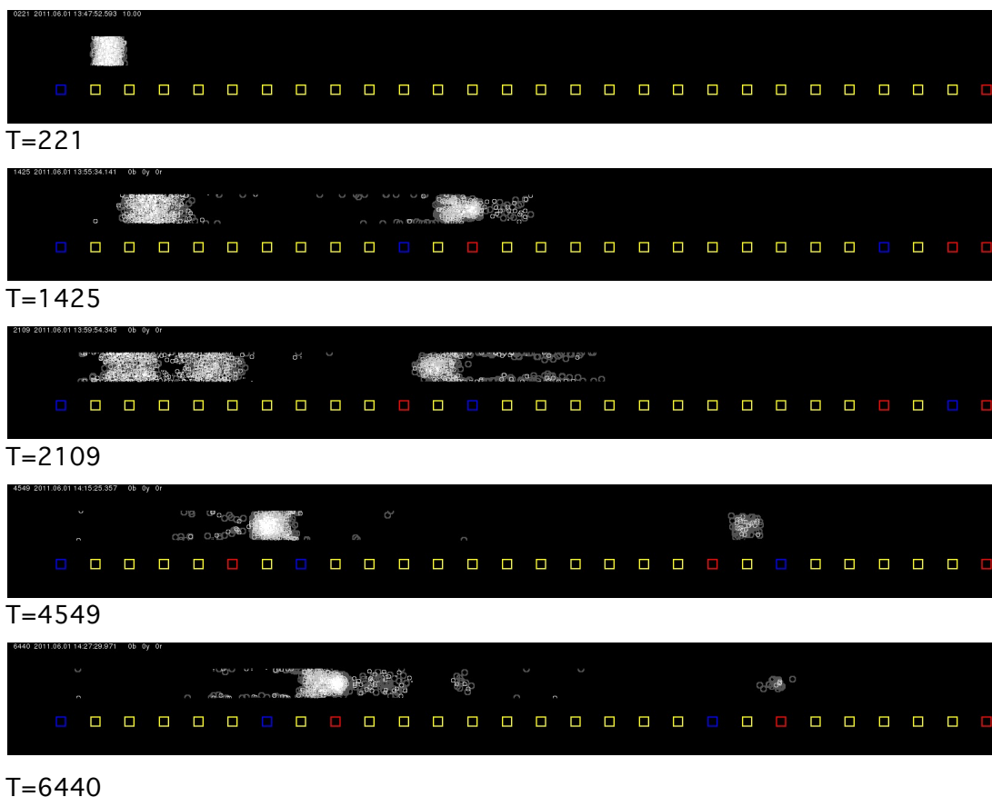
Fig. 12 Simulated separation of DNA with small (1%) mobility differences by feedback modulated local electrophoresis.
