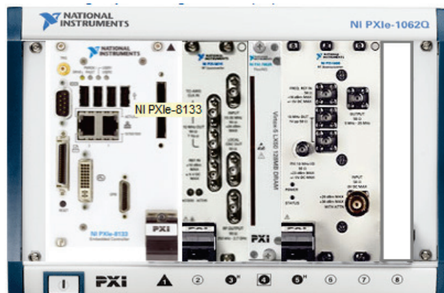
Figure 3-31. PXI 2.7GHz up- and downconverter with NI 5600 and NI 5610
