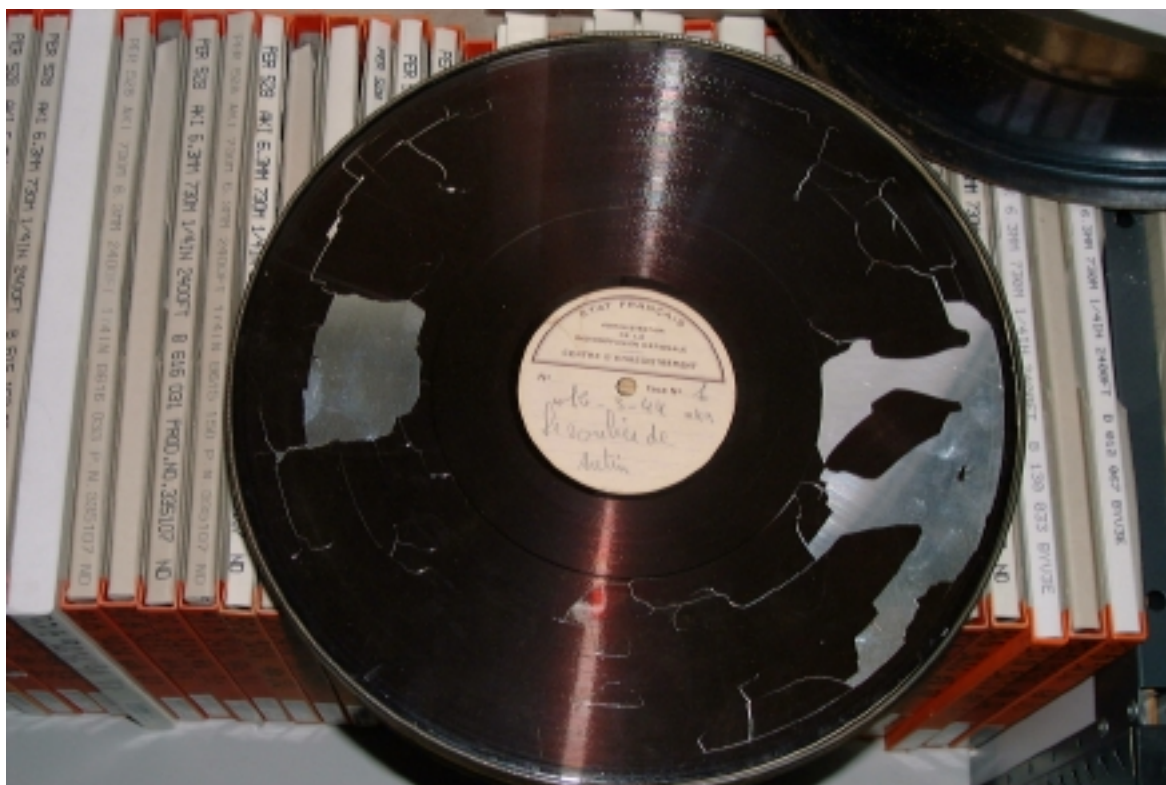
Exhibit 11 Aluminium coated record with a valuable recording of a theatre work by Cocteau, technically irrecoverable
