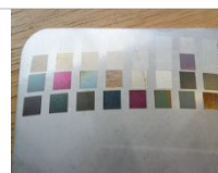
Stainless steel, Pulse duration: 4-200 ns.
