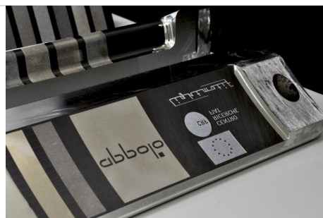
Engraved logos on the mould surface.
