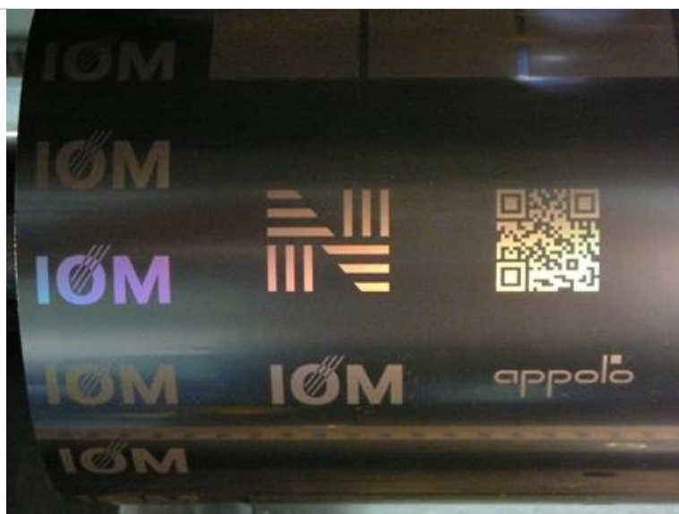
Photograph of a machined sleeve with decorative patterns.
