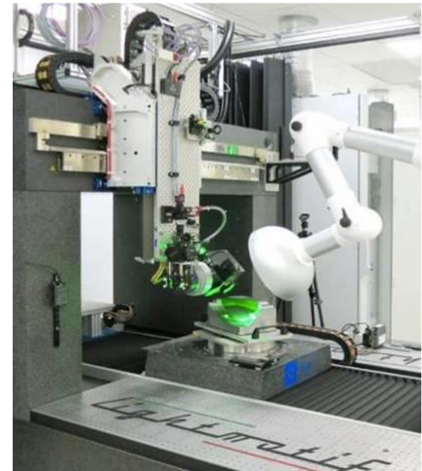
The machine developed in the FP7 project NANOCLEAN in process of structuring the demonstrator mirror cup mould.
