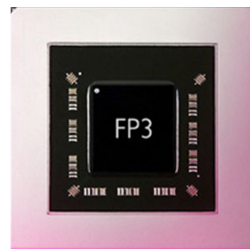
Example 3: Alcatel Lucent 400G network processor
