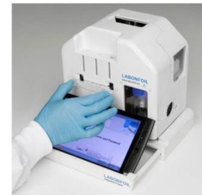
SmartCard lab-on-a-chip device for real-time PCR detection of food borne pathogens, marine algae analysis, climate change and Colorectal Cancer patients monitoring (LABONFOIL Project)
