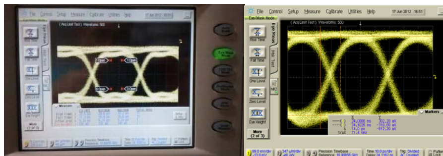
Fig. 2.5.2-2: Input and output eye diagrams at 25 Gbit/s (left and right panel, respectively)
