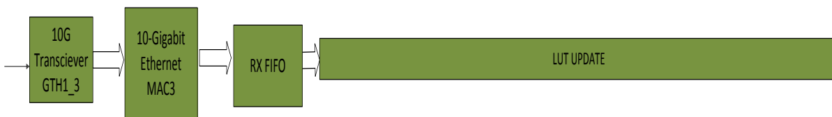
Figure 3-17: GMPLS-to-node Link Layer 2 Function Block Diagram
