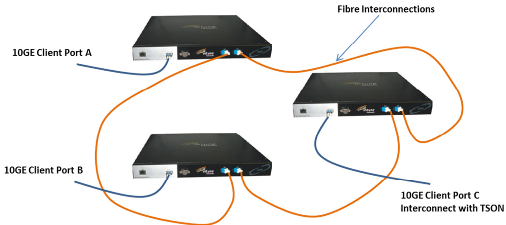
Figure 3-1: OPST Beta node configured for 2 test traffic ports and 1 TSON interconnect port
