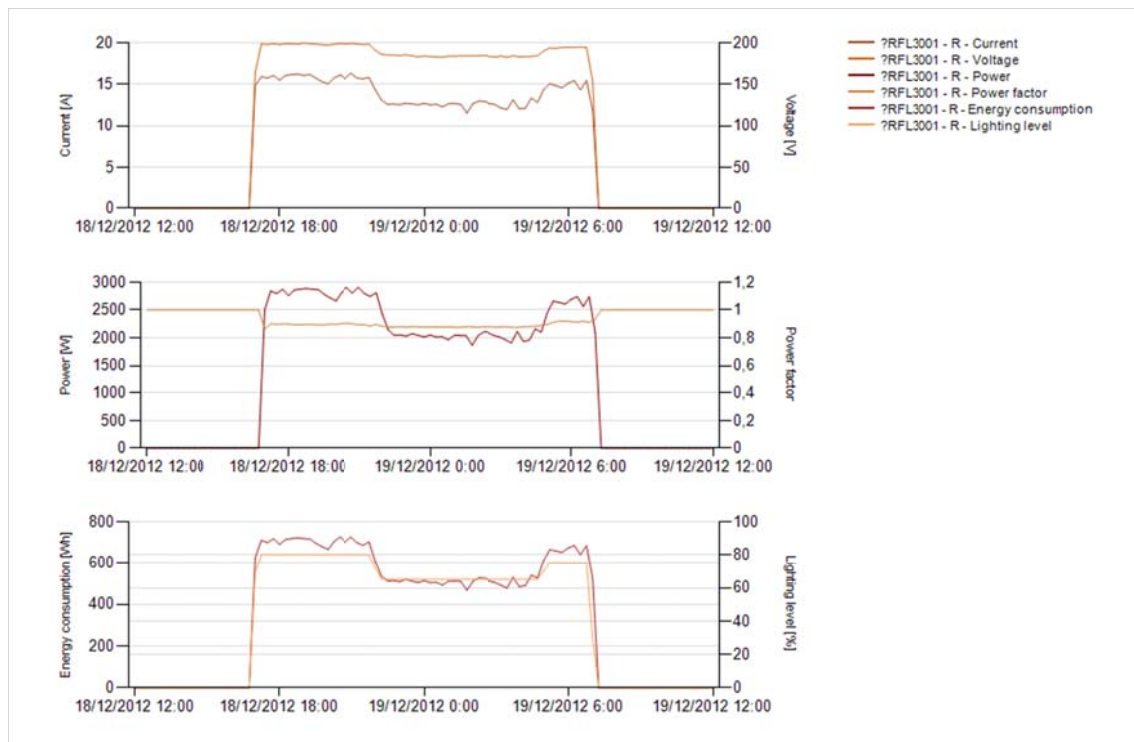
Figure 13: Calendar-based regulation on a real device in Alginet
