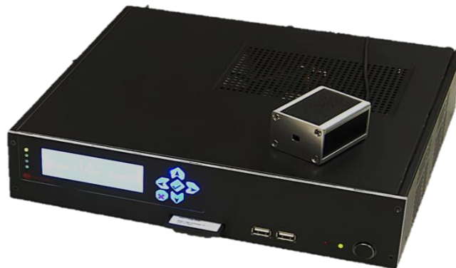
Figure 23 DIOMEDES hardware demonstrator used for the processing of the 5.1 to 2.0 downmix
