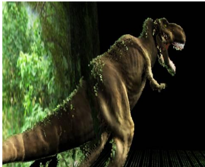
Figure 8: From an extreme angle, the individual points are clearly visible. Filling the place in-between results in false geometry added to the scene. Filling the space with bigger points gives a more pleasing result.
