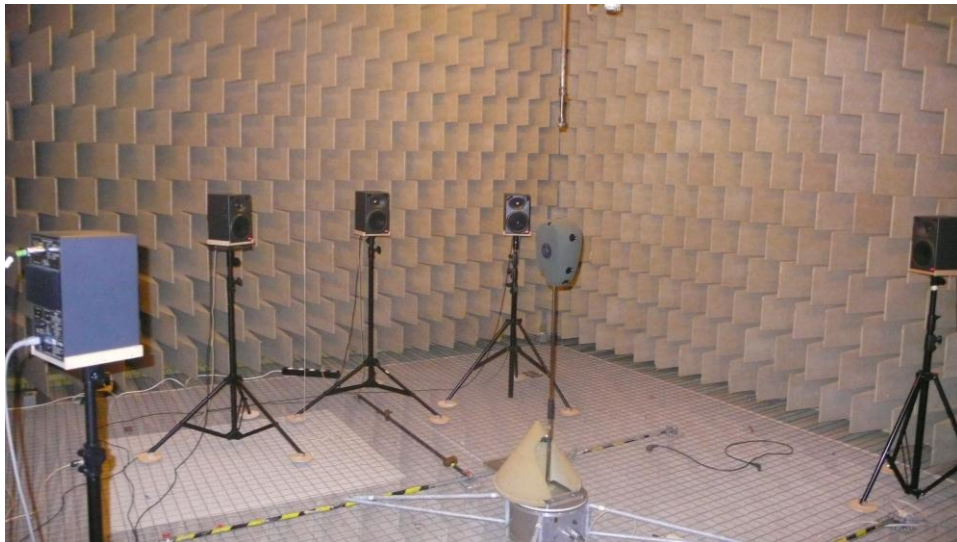
Figure 29 Measurement setup in the anechoic chamber
