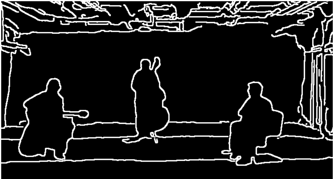
Figure 5: Classification of image pixels into edge and non-edge areas
