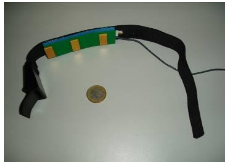
Figure 12: An ecological EMG band for wearing on arm or leg (www.infusionsystems.com)
