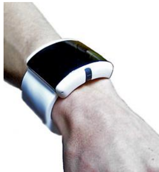
Figure 10: Pulse Wave Velocity Measurement of Blood Pressure ( www.exmocare.com )
