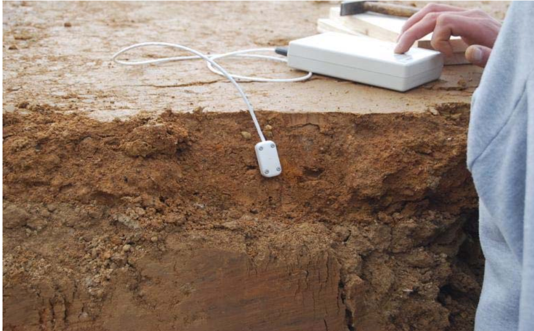
Figure 21: Field measurement with the KD2Pro device in one of the test sites
