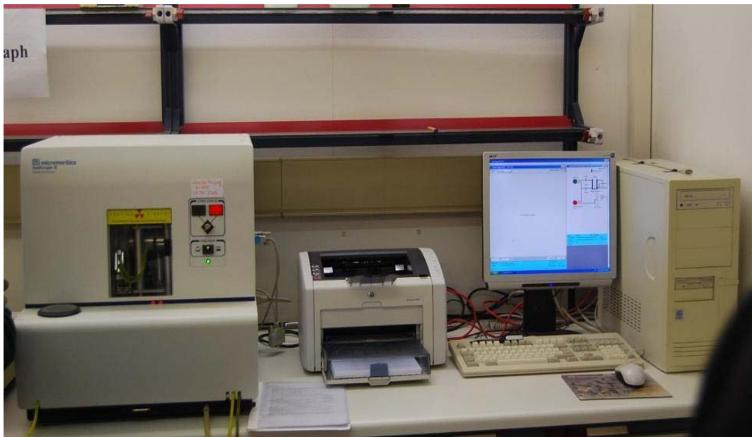
Figure 18: SediGraph – measurement instrument for measuring soil texture (grain size distribution)
