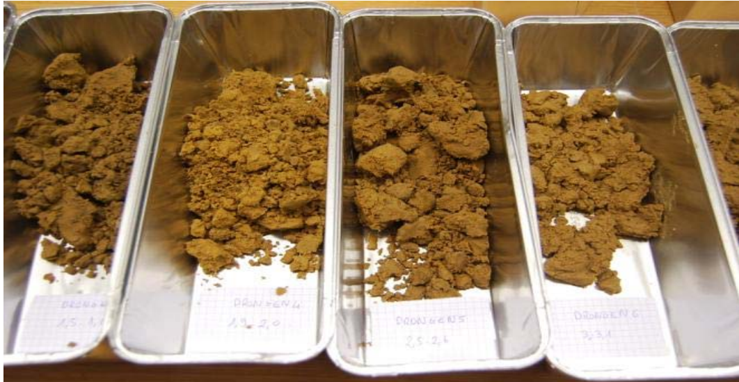
Figure 17: Soil samples drying for preparation
