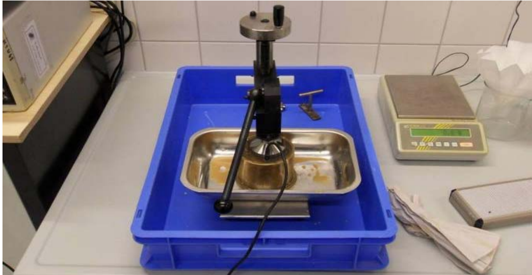
Figure 19: TK04 – measurement instrument for measuring thermal heat conductivity
