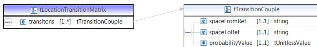
Figure 21: Location transition matrix schema
