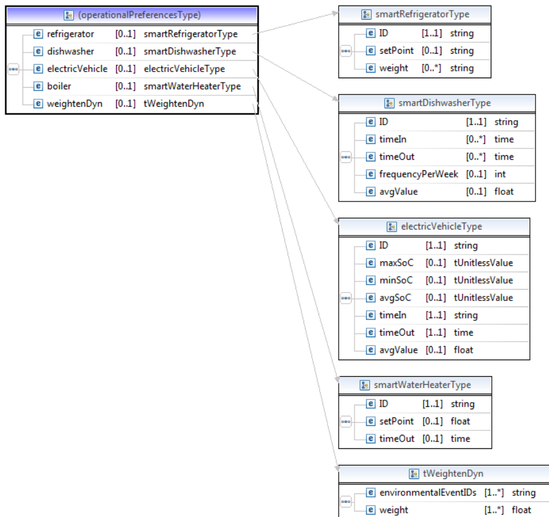
Figure 32: Operational preference with modelled devices XSD specification
