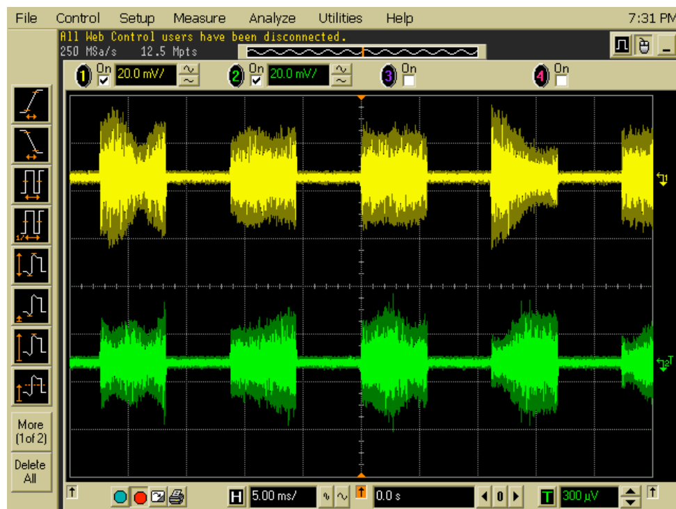
Figure 6-31: Spectrum analyzer plot of the IF signal at the output of the RF Downconverters + SAW SMD filter.
