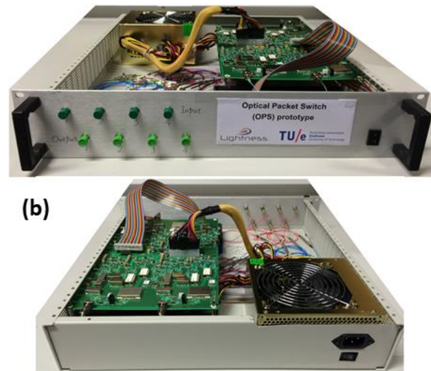
Figure 5.1: (a) Modular OPS architecture with distributed control. (b) OPS prototype
