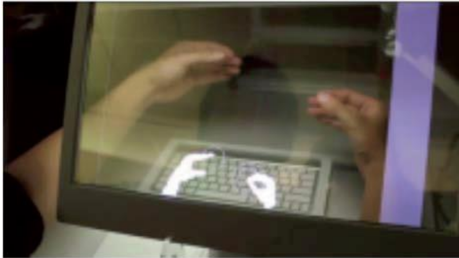
Figure 7. A Kinect-driven prototype desktop environment by the Microsoft Applied Sciences Group allows users to manipulate 3D objects by hand behind a transparent OLED display ( www.microsoft.com/appliedsciences )
