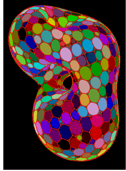
Fig. 4. Intersecting the surface with a HCP grid. The patches (random colorization) consist of two parts: The bright ellipsoid regions are direct intersections of the surface with a virtual sphere in the HCP grid. The dark regions around them still relate to the same node, but in the sense of proximity similar to a Voronoi diagram. We marked the borders between the patches in red and intersections where more than 2 neighbors meet with green pixels.
