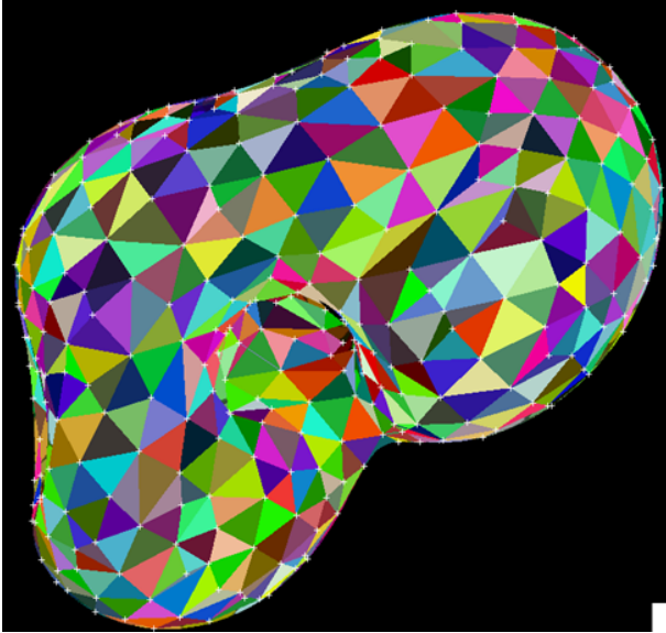
Fig. 8. Triangulation of the reference points. The imposed heuristics produce a complete, non-overlapping triangle mesh between the reference points in parallel, which leads to extremely fast computation.
