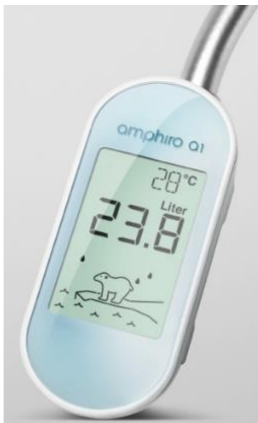
Figure 2: DAIAD@feel prototype with display only. The product is commercially available named "amphiro a1 basic"
