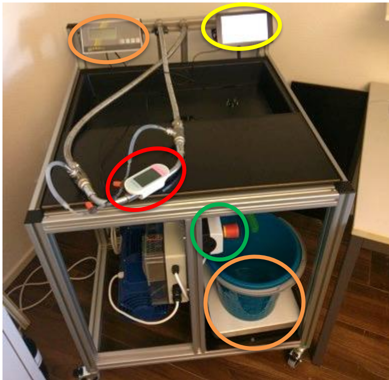
Figure 11: Front view of the newly developed test system. The touchscreen (yellow) is used to control the flow rate and valves of the test system. The emergency switch (green) can be used to deactivate the whole system in case of technical failure. The accuracy of the DUT (red) can be measured using a high precision scale (orange).
