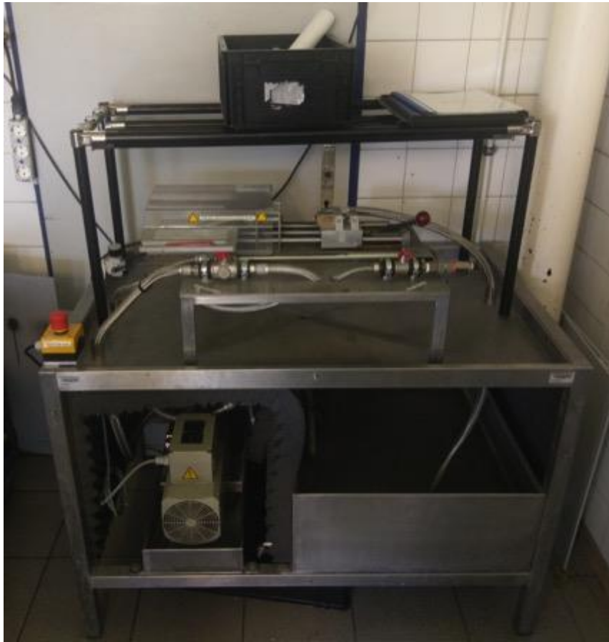
Figure 18: Calibration equipment at production site. The device is calibrated and tested with a water-flow similar to real water extractions.
