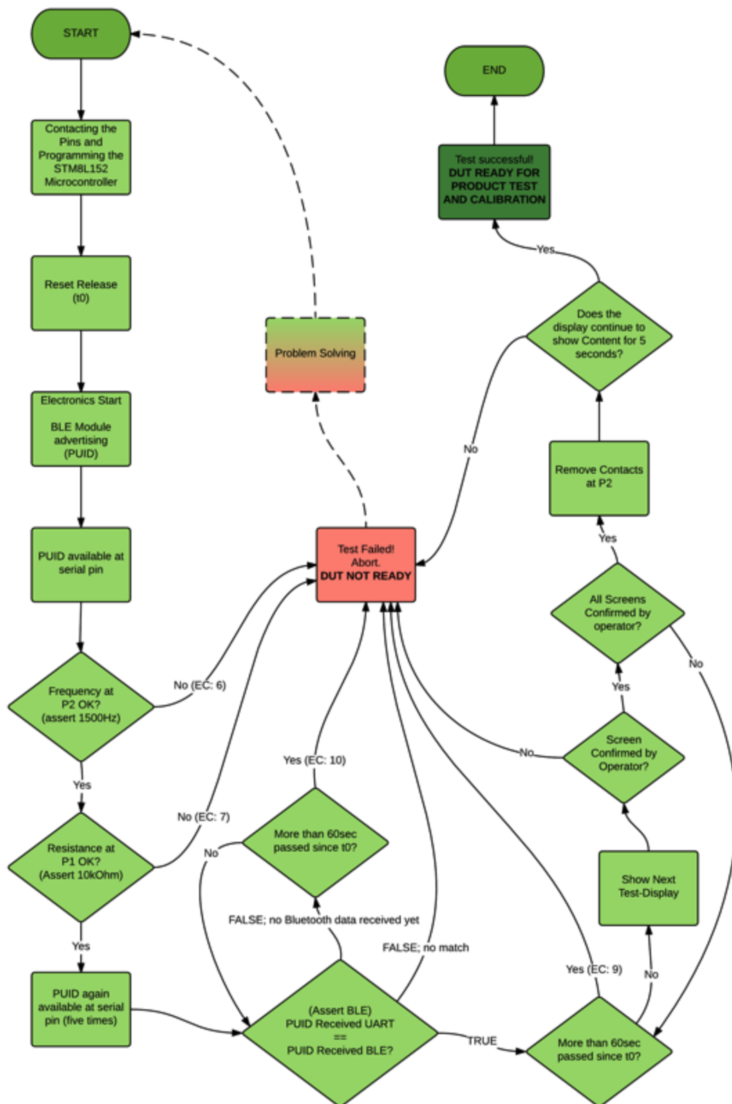
Figure 16: Flow chart of testing procedure in production
