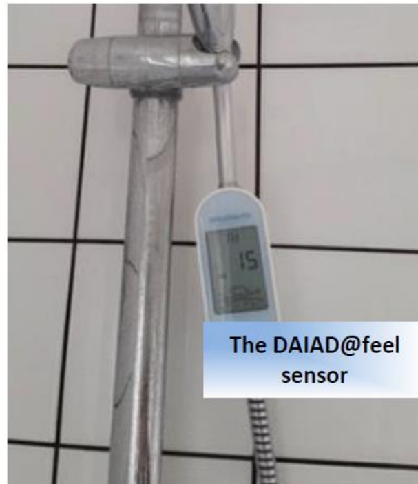
Figure 8 DAIAD@feel prototype mounted in a shower.
