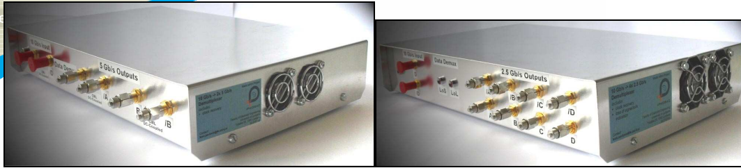
Figure 34 Photographs of the manufactured 10 to 2x 5 Gb/s (lefthand side) and 10 to 4x 2.5 Gb/s (righthand side) data demultiplexers.
