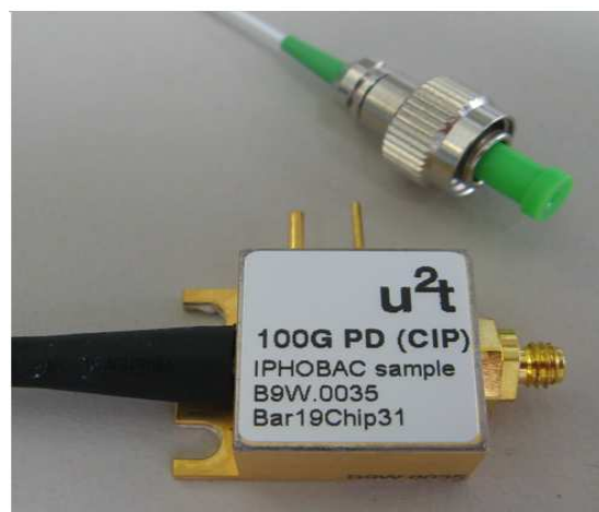
Figure 12 Photos of the packaged photodiode chips from UDE (top left) and CIP (top right) and the corresponding packaged photodetector modules (bottom).
