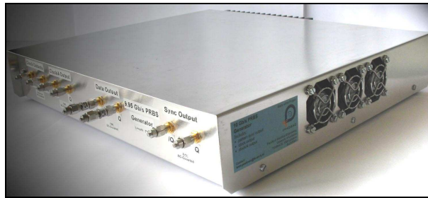
Figure 33 Photograph of the manufactured 10 Gb/s PRBS generator.
