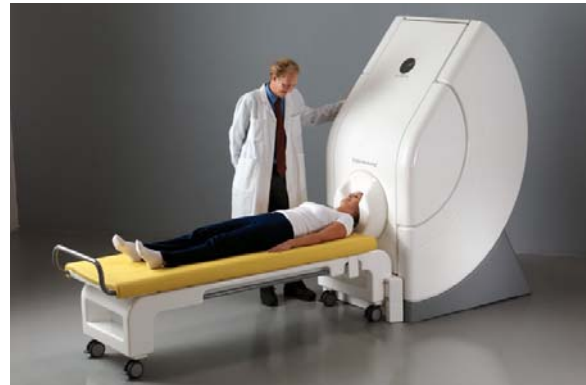
Fig. 3.3-3. Commercial LT SQUID MEG system providing sophisticated 3D mapping of brain activity, (courtesy of [3.3-24])
