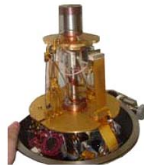
Fig. 3.2-3 Photograph of the RSFQ DSP cryopackage mounted on Sumitomo RDK-101DP cryocooler. The system supports DC bias of a total 2.5 A, up to 40 Gbps I/O channels, and 40 GHz clock lines.
