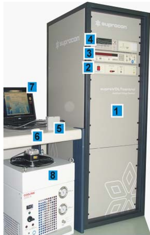
Fig. 5-7. The cryo-cooled Josephson voltage standard, fabricated ad Supracon AG. The system consists of the following components: 1: pulse tube cooler with a SIS Josephson junction array and the 75 GHz microwave electronics installed in the 19" rack, 2: control electronics, 3: source looking counter, 4: null detector, 5: 3-channel polarity reversal switch, 6: sensors for temperature, pressure and humidity, 7: computer control, 8: 2 kW compressor unit.
