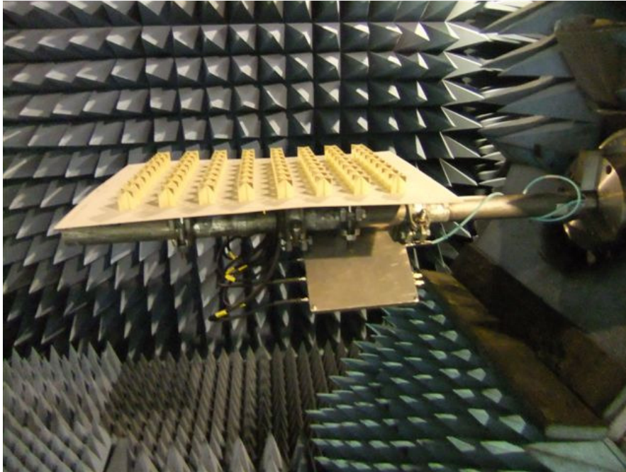
Figure 7-4: BuNGee multi-beam HBS antenna undergoing trials in CASMA’s anechoic test chamber.
