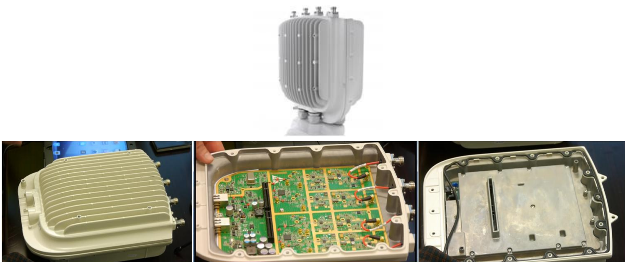
Figure 7-1: Small cell (Access BS) technology – housing, RF module, modem part (shielded)
