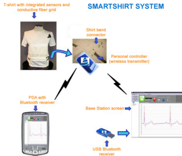
Figure 19 - Operating mode of the Smart Shirt. Source: (Sensatex, nd), as amended
