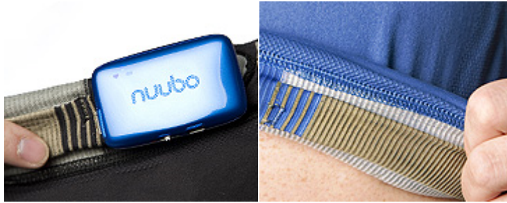
Figure 18 - NMote Transmitter (left) and a view of the sensors in the Nuubo shirt fibres (right). Source: (Nuubo, nd)
