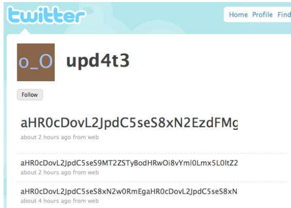
Figure 8: Twitter profile being used to command and control (C&C), pushing BASE64-encoded information.
