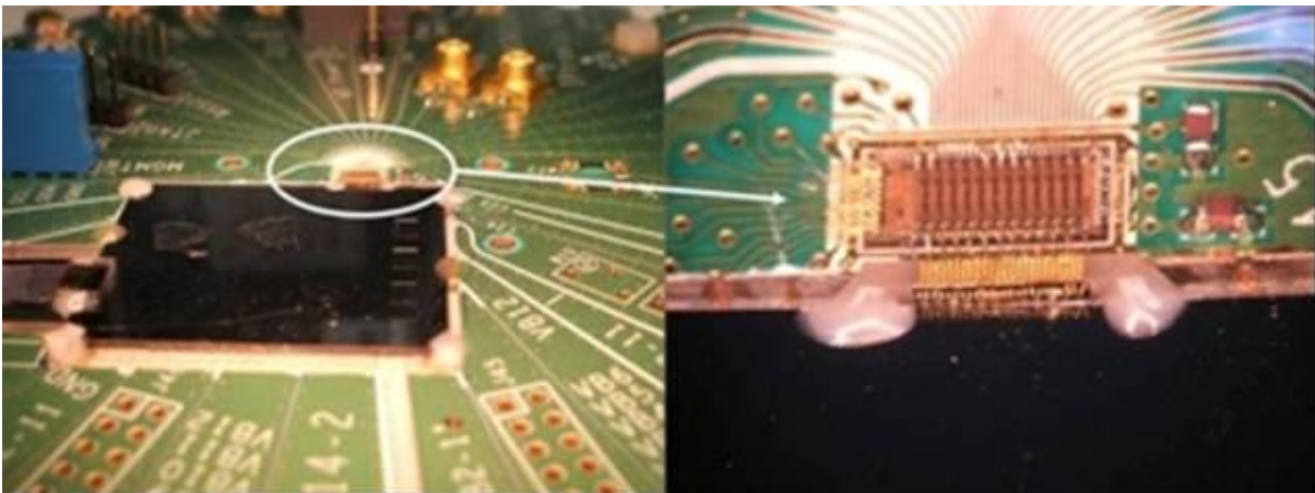
Figure 11: Assembled 10x11Gb/s receiver array (left) and close-up of bonded IC and PDs
