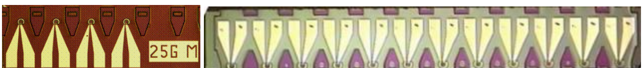
Figure 4: Photodetector arrays fabricated: 4x28G (left) and 10x11G (right)
