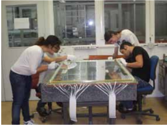
Figure 3. Stretching the fishing-line spacer in a zig-zag pattern.
