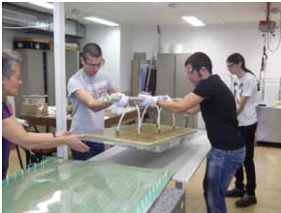
Figure 4. Using a vacuum system, a glass plate is lifted in order to be placed on top of the previous one.
