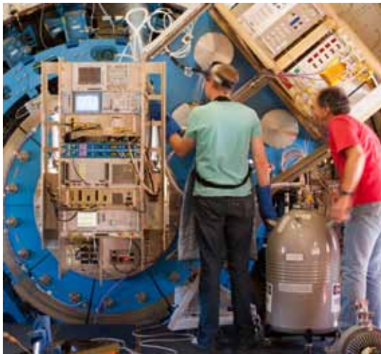
Figure 3. The detector GREAT and the telescope counterweight at the aft of the telescope while filling up with liquid nitrogen.
