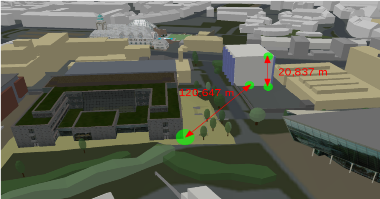
Figure 6: Conceptual view of the measuring tool. The red arrows indicate the distance to measure of the 3D points selected. 3D spheres on those endpoints indicate the 3D perspective distortion. A point closer to the viewer will be surrounded by larger spheres as a point far away. With this a user can easily verify the expected results. This should assist the user as the points selected are not on a simple plane but in 3D space. As an example, the first measurement (left in image) shows the distance between 2 buildings where the second building is not as close to the viewer as the first one. Therefore the sphere is bigger on the first building. When using a frontal perspective, for example the measurement of a building's height, both spheres should be of the same size as shown in the measurement on the right side of the image.
