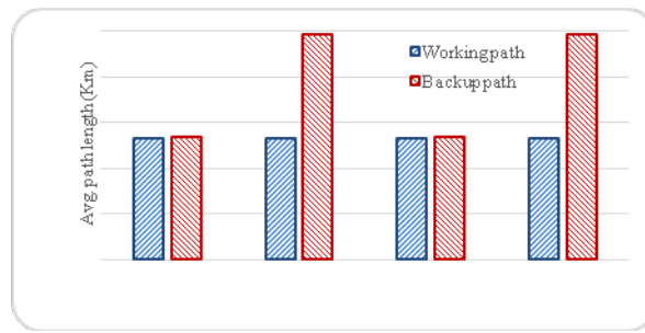
Figure 20: Average path lengths for dual-homed and baseline architecture using DPP-DH-W and DPP-DH-L for 27 Tbit/s total network traffic
