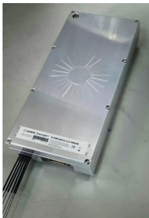
Figure 7-3 a) A 48-fibre single-sided optical switch module using a single board ASIC-based controller; b) Detail of the controller card showing the IMEC-developed Polatis DirectLight driver ASICs
