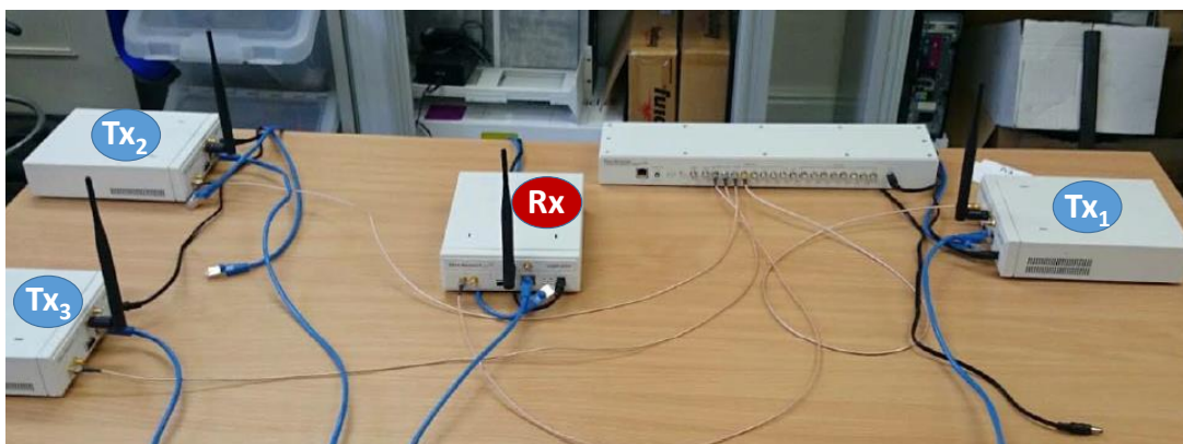
Figure 2.14: USRP hardware test set-up.
