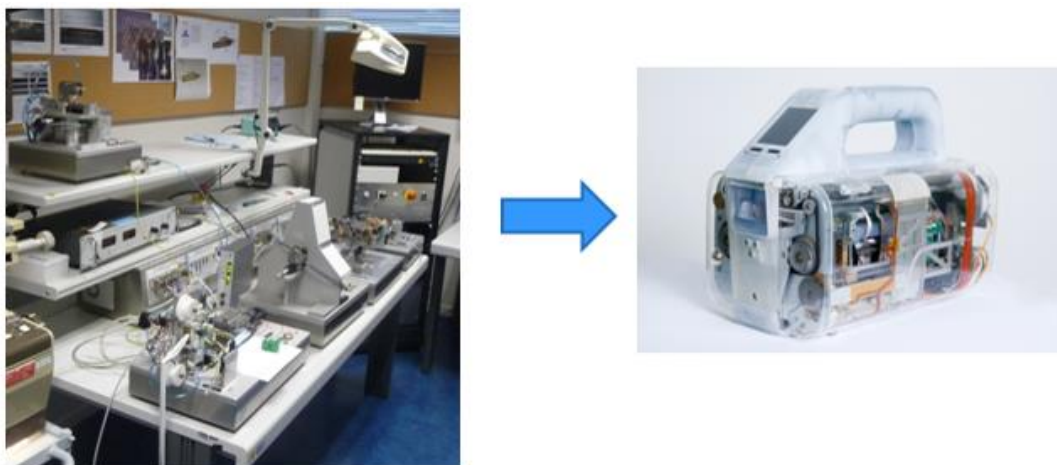
Figure 22 : The VECTOR processes were evaluated using table top stations and their results needed to be integrated into a hand-portable tool.
