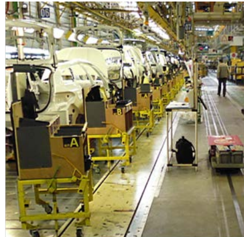
(Left) Kit preparation in the kitting supermarket (Right) Kits delivered and synchronized with the production line
