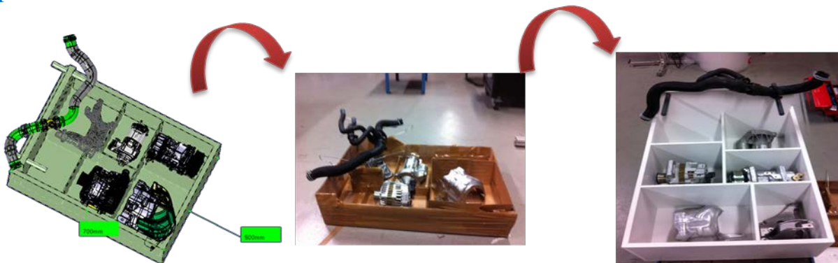
Iterative design of the kitting box (2 nd iteration)
