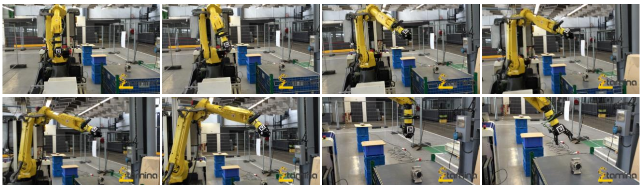
Figure 29 shows the result of a bad registration: The pose of the object is computed wrongly, and the robot arm approaches the object from the wrong direction.
